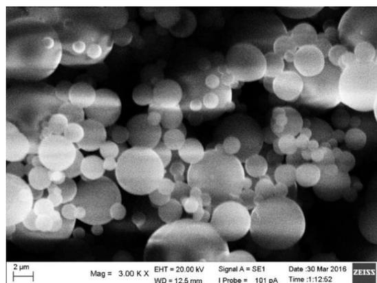
**Figure 1. Morphology of dry powder of nanoparticles using *Electron Microscope (SEM)***
